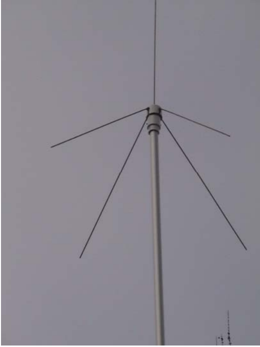
Home-built 2-meter antenna
